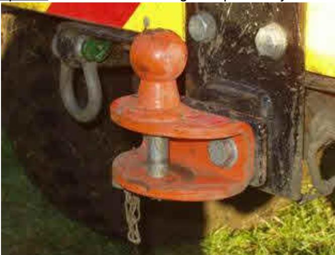
10mm plate. This was purposely designed to sustain the extreme forces applied to it during severe recovery exercises.
