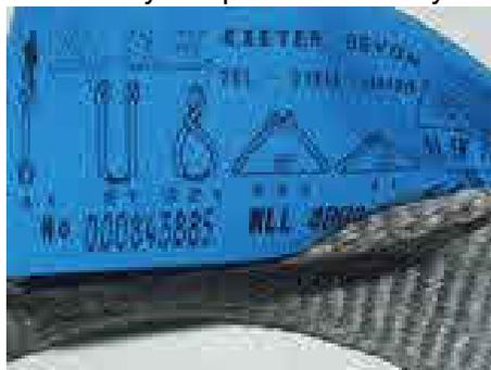
attached to it showing what it has been designed and tested to pull. Here is a photograph of the label you should expect to find on quality strops. The strop in the photograph has been rated at different rates dependent on the configuration in use. Always check the configuration loading before you actually use it.
